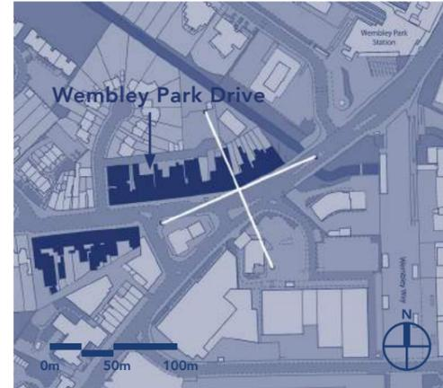
The footprint of the proposed tower is overlaid onto the existing urban condition. The tower is positioned just off the Wembley Way axis, centred over the Wembley Park Drive area. Two of the housings for the four lasers land on traffic islands and the other two in car parks.
